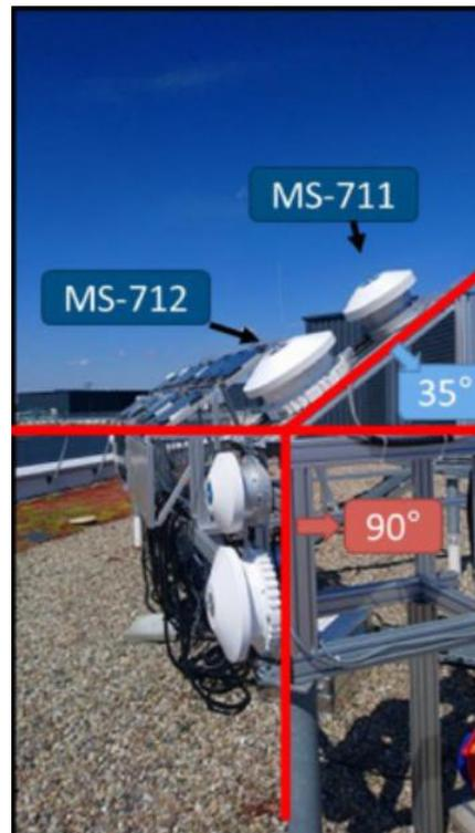
**Figure 1** Picture of the installation of two sets of spectrometers MS-711 and MS-712 at two different tilt angles: 35° and 90°.
