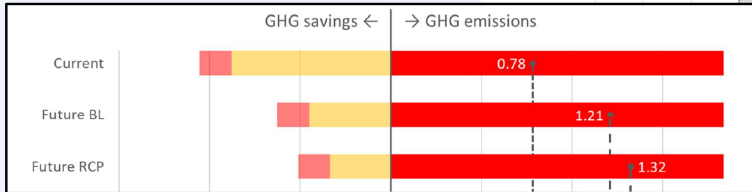
Fig. 4. Process contribution analyses of GHG footprints for treatment of 1 kg in year 2030. Numerical values are provided in Supporting Materials 2. Net GHG footprints for each scenario are indicated with grey/white squares. Emission saving potentials are indicated with grey bars. The GHG savings from avoided fossil CO 2 emissions at HVC end-of-life are marked with a dashed border. These savings are to be subtracted from the results in case one assumes a use and end-of-life scenario for the HVCs or products derived in which incineration is not the end-of-life fate. GHG: greenhouse gas; BL: baseline scenario; RCP: representative concentration pathway 4.5 W/m 2 by 2100 scenario; EB: electric boiler; BB: biogas boiler; CO 2 : carbon dioxide; HVC: high value chemical.
