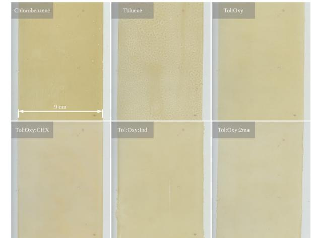
Figure S17: Images of PCBMs dry films deposited by slot-die coating a 5 μm wet film on bare PET substrate, using 10 mg ml<sup>-1</sup> inks with solvent systems of either chlorobenzene, toluene, toluene:O-xylene (7:3v/v) (Tol:Oxy), toluene:O-xylene:cyclohexanone (6:3:1v/v) (Tol:Oxy:CHX), toluene:O-xylene:indan (6:3:1v/v) (Tol:Oxy:Ind), toluene:O-xylene:2-methylanisole (6:3:1v/v) (Tol:Oxy:2ma).
