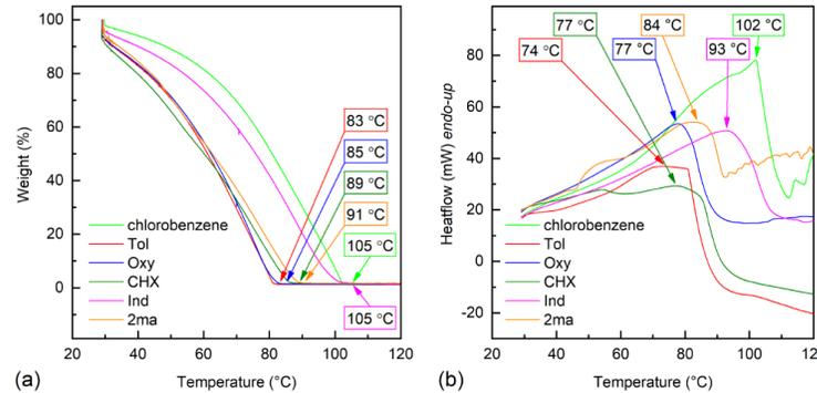
Fig. 6 Simultaneous Thermal Analysis of PCBMs inks with various solvent blends at 10 °C per minute. The labelled temperature on the gravimetric analysis is when the weight derivative with respect to time is equal to zero (a). The labelled temperature on the thermal analysis is the peak heatflow (b). Solvent system abbreviations are Tol = toluene, Oxy = O-xylene, CHX = cyclohexanone, Ind = Indan, 2ma = 2-methylanisole.
