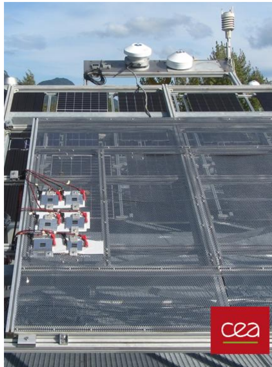
Figure 4. CEA set up for outdoor monitoring.
